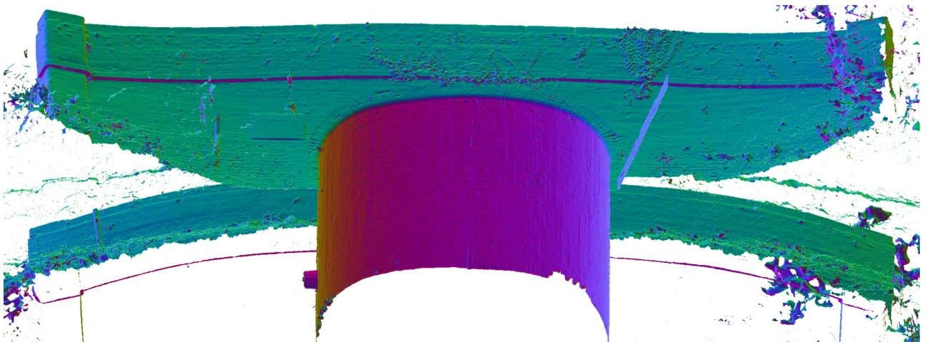
Figure 20: This inclined view has each point coloured with a mix of red, green and blue depending on the normal direction. Changes of angle and surface roughness are highlighted.
