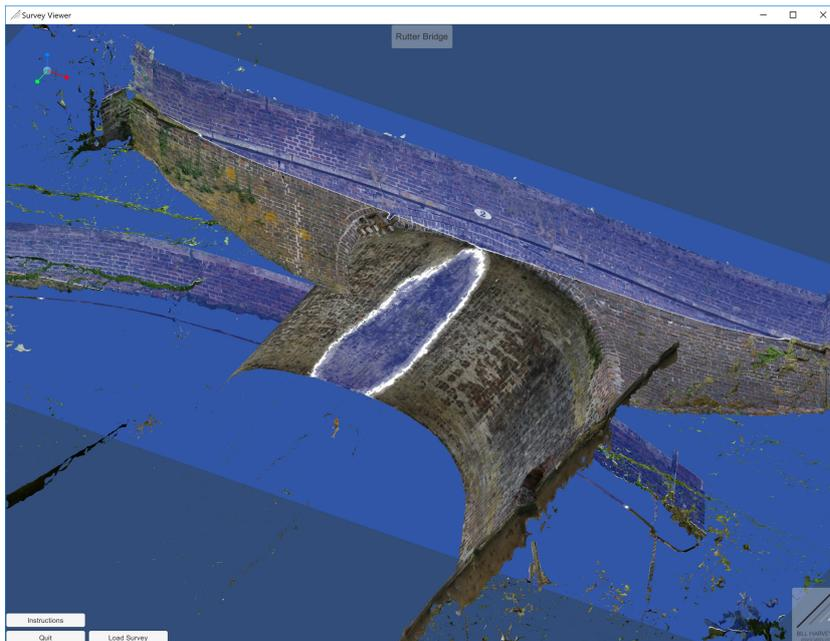
Figure 7: Orthographic view of model with horizontal plane. The plane was created by right clicking on the model, selecting "Horizontal Through Point", and defining the point at the near side crown.
