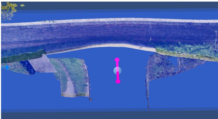
Figure 28: Two parallel vertical planes demark a slice.
