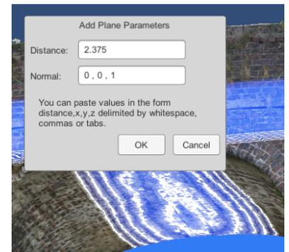
Figure 19: Specifying a plane with a normal and offset from origin.
