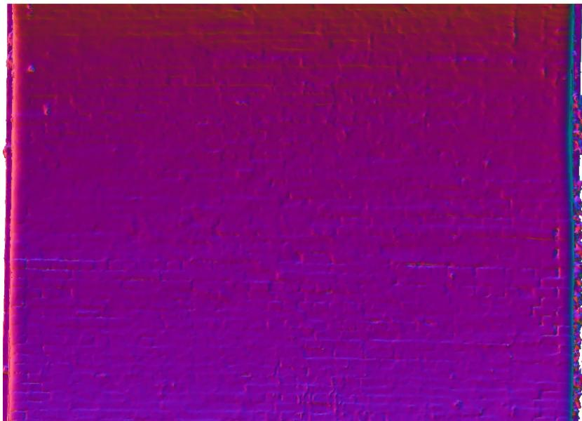
Figure 24: To clean the image a bit we put in a cut plane and removed everything below it. That takes out the ghost of the towpath edge and made things clearer. Notice the thin bright stripe where there is a drop between bricks near the crown at the left. The model is tilted here to emphasise that.
