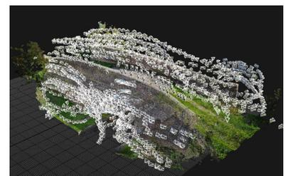
Figure 5: Position and orientation of each photograph used in constructing the model.
