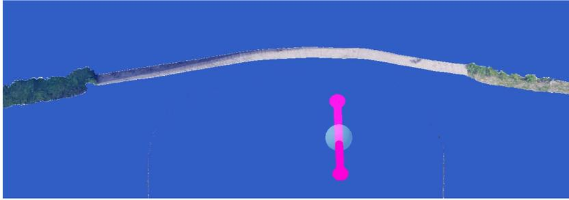
Figure 29: Clipping at both planes in opposite directions isolates a strip.
