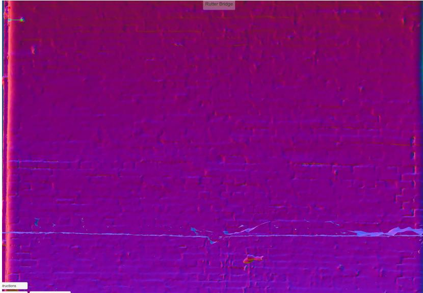
Figure 23: Tinting every bit of surface according to the direction of its normal emphasises empty joints and other damage. Is it just me or do the colours change across a diagonal?
